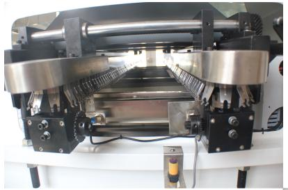
1.Input device:Corrosion resistant, not deformation of titanium claws
