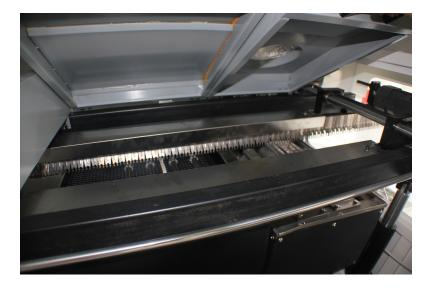
3.Conveyor part: Guarantee the PCB is complete, welding and transport
